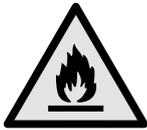
**WARNING:** Danger of fire / flammable materials. This symbol is located on the compressor and indicates the danger of flammable materials. Do not remove the sticker.
